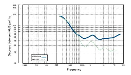
All the polar measurements were taken using calibrated MLSSA test equipment, with a microphone placed at a distance of 9 metres from the rotational axis of the loudspeaker enclosure under test. This method reduces the effect that the interaction between the MF and the HF has on the measurements.
